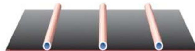
On sheet metal soldered tubing system
